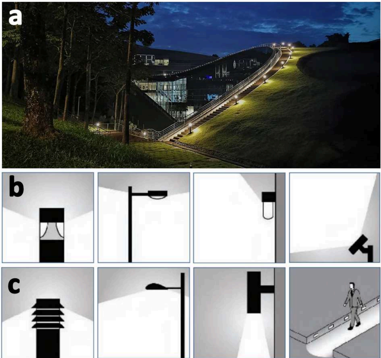
Figure 18. (a) Uplights that line the roof of the ADM building could disorient the birds. Photo credits: William Yung. (b) Examples of uplight that should be avoided. (c) Examples of designs that minimise light spills, which do not require removal of the light or compromise public safety. Figure credits: San Francisco Planning Department, 2011.
